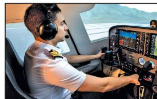
The ALSIM AL172 MKII flight simulator represents a Cessna 172SP Skyhawk NAV III aircraft equipped with the Garmin 1000 avionics suite, meeting the requirement as both FAA FTD level 5 and EASA FNPT II for maximum credit hours. (Courtesy ALSIM)
